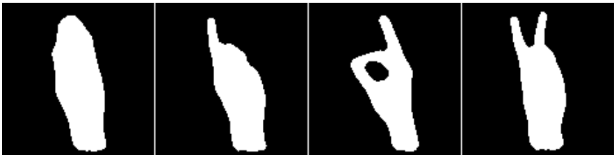
Fig. 8.3.1 Predefined static gestures recognized by the system during tests
