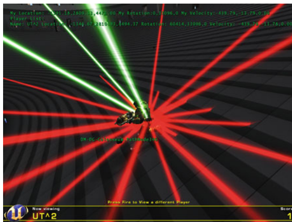
Fig. 5.3 Ray-Tracing Level Geometry Sensors. Gamebots has a debugging option for viewing ray traces on a bot. The figure shows all 22 ray trace sensors around the bot, with the contrast heightened to improve visibility. Some of the rays aiming upward are brighter because they are not colliding with any level geometry. These sensors provide the bot with information about the structure of its immediate environment, which helps it reason about how best to dodge enemy attacks. Though disabled in BotPrize 2010, these sensors should help the bot be more aware of its surroundings in future competitions
