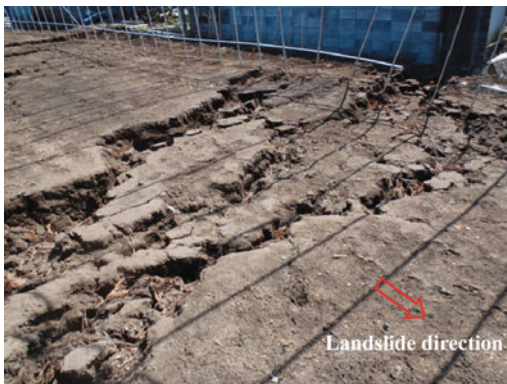
Photo 30.2 Fractures are located 5 m from slope shoulder opening width: 0.3 m, vertical offset: 0.2 m
