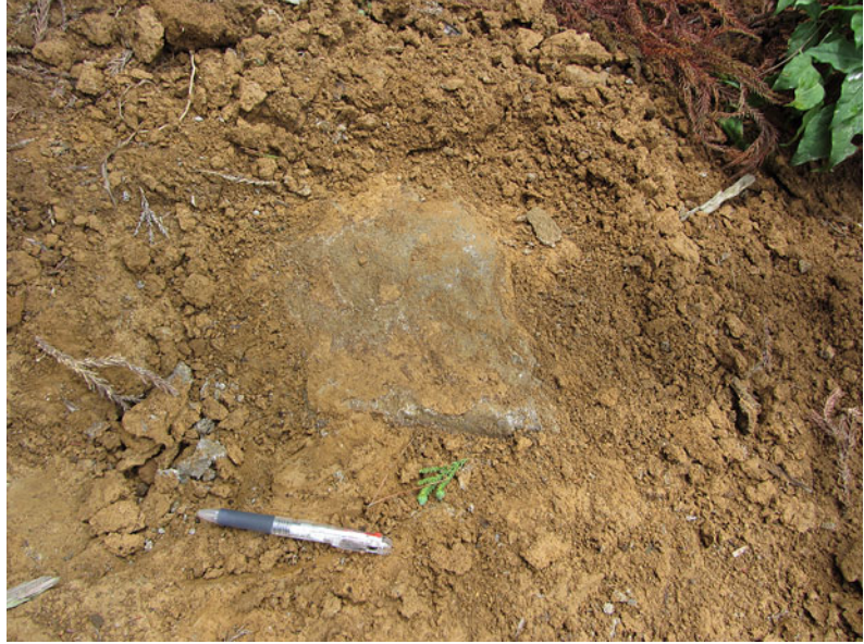
Fig. 73.3 Stone pieces in the slip surface
