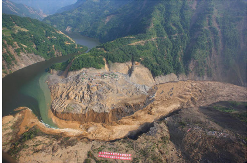
Fig. 98.1 Looking downstream, shows flow in the channel of the Tangjiashan natural dam shortly after breaching ( http://blog.gxnews.com.cn/u/4332/a/147392.html )
