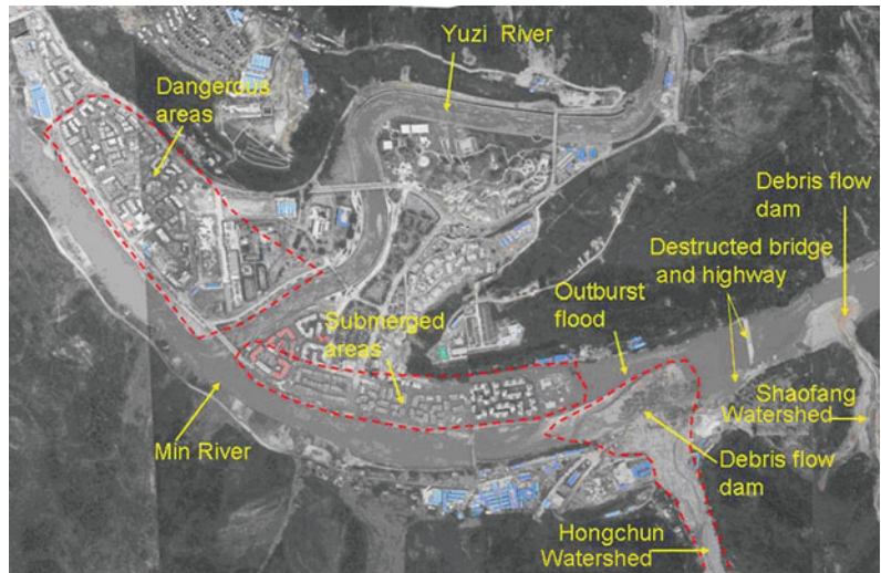
Fig. 106.7 Yingxiu Town endangered by 8.14 debris flows and outburst flood of dammed lakes
