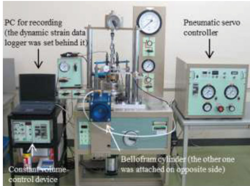
Fig. 47.10 Cyclic ring shear test system
