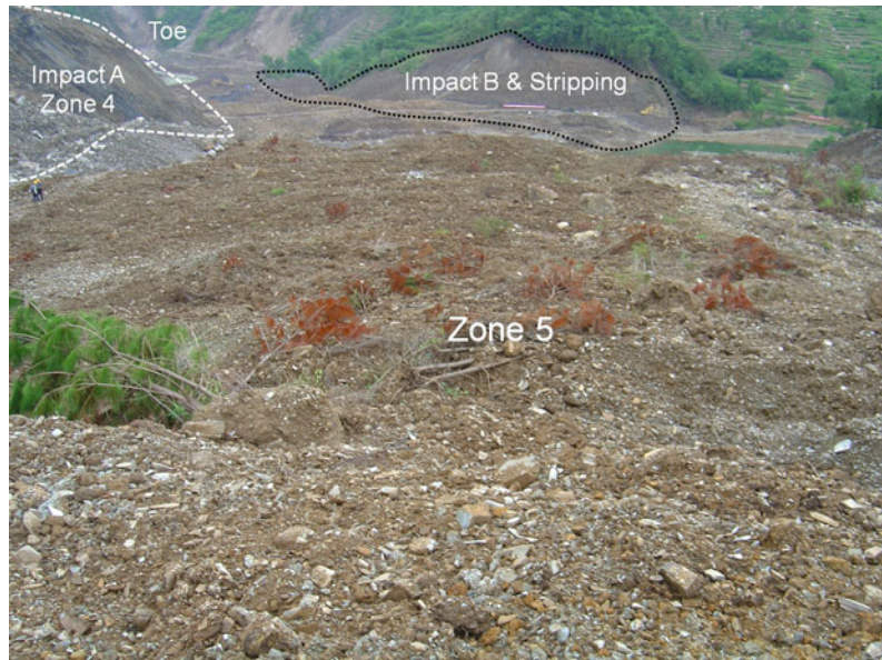
Fig. 51.5 Impacts A and B and stripped surfaces, downstream debris flow and deposition and toe of Donghekou rockslide-debris flow
