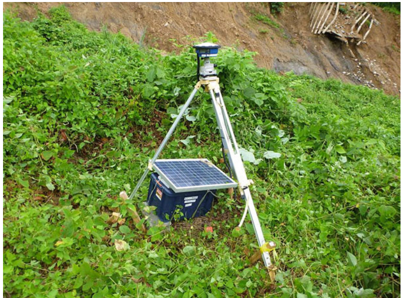
Fig. 35.3 GPS observing station
