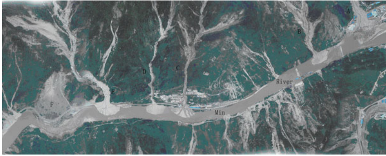
Fig. 106.5 Debris flow and the following hazards change river channel (Yingxiu to Laohuzui). a. Hongchun Watershed, b. Shaofang Watershed, c. Xiaojia
