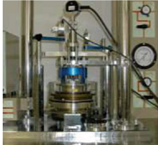
Fig. 47.3 Ring shear test apparatus used
