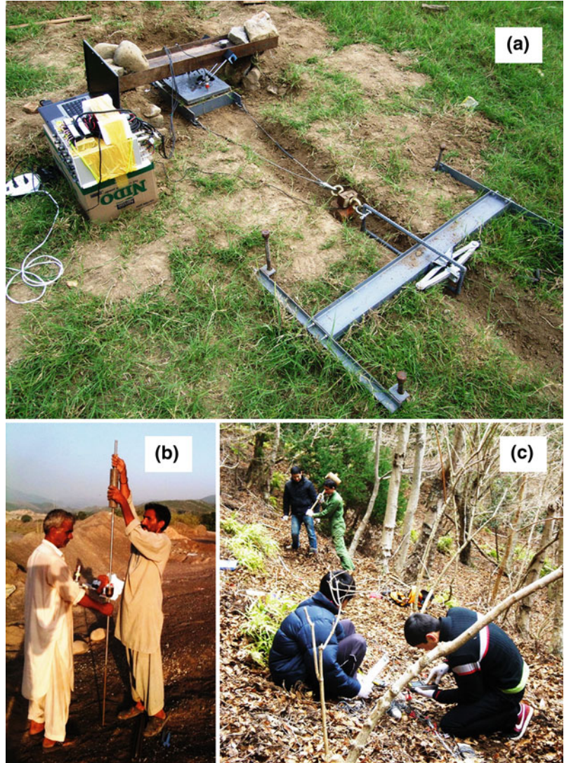
Fig. 95.3 Field tests. a Field direct shear. b Portable dynamic cone penetration. c Seismic refraction
