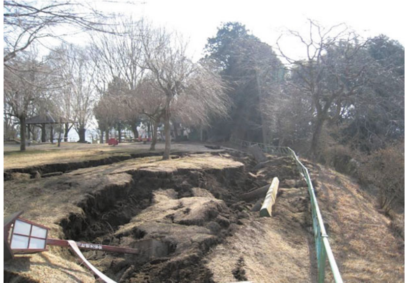
Photo 33.1 Slope displacement induced by the 2011 off the Pacific coast of Tohoku Earthquake (BB' cross section)
