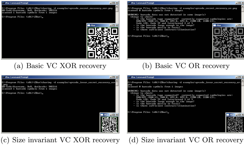
Fig. 9. Attempted authentication of each of the barcodes based on the type of secret recovery used
