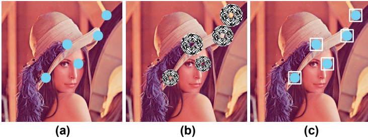
Fig. 3. This figure shows (a) the original Lena image with its SIFT features shown as circles, (b) watermark patterns that will be embedded around the SIFT features, and (c) watermarked image and its extracted SIFT features shown as rectangles with SIFT features of the original image shown in circles. We show only five SIFT features that have the top-five highest strength values.
