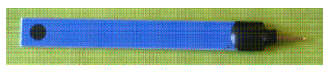
Fig. 2. Modifiable screen-printed carbon electrode for determination of dopamine and explosives in aqueous solutions
