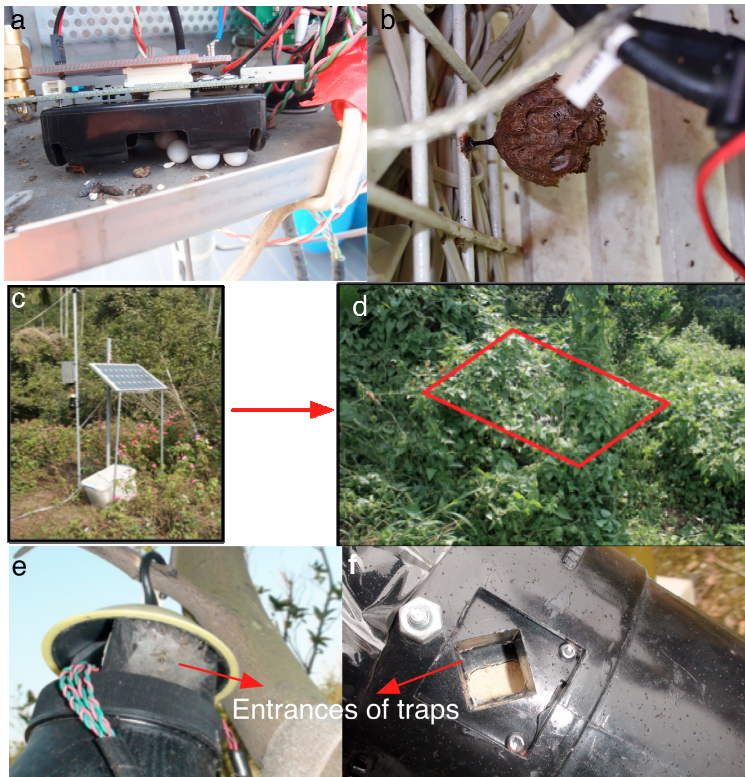
Fig. 6. The problems that WSNs encounter in wild areas [3-4]. (a) the intrusion of geckos, and they laid eggs near the sensor nodes inside the waterproof protection case; (b) a beehive is built inside the waterproof protection case, which implies that the activity of wild bees is present in the case; (c) The initial deployment scene of the solar panel used to power the sensor node; (d) The scene after the monitoring system has been deployed for one year, and the solar panel was covered by these thick leaves; (e) Entrance of the pest trap equipped with automatic infrared sensors is cobwebbed, which prohibits the pests (for the oriental fruit fly) from being attracted into the trap; (f) Entrance of the pest trap for the tobacco cutworm is jammed with the beehive.
