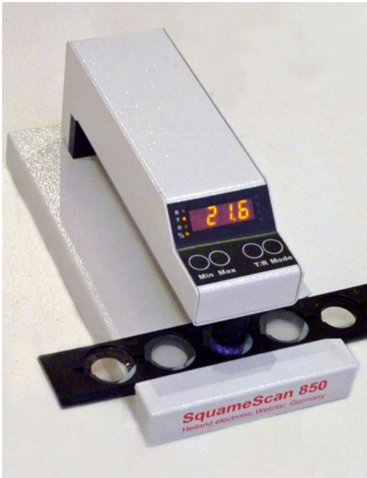
Fig. 28.2 The compact infrared densitometer SquameScan 850A with an inserted sample applicator [16]
