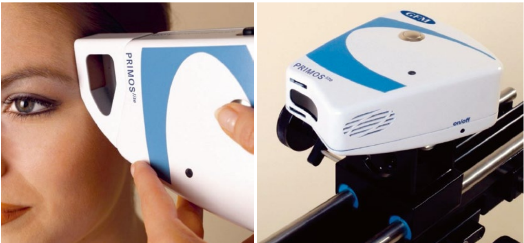
Fig. 4.13 Example of a compact, pico DMD-based sensor in mobile measurement ( left ) and on a stand ( right ) (Photos: GFM)
