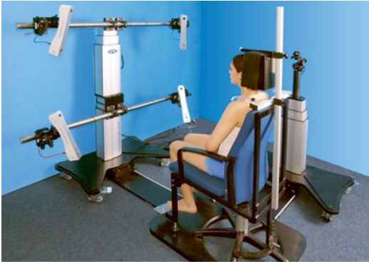
Fig. 4.14 Biomedical body scanning station with four sensors and recallable precision positioning for 180° scanning (Photo: GFM)
