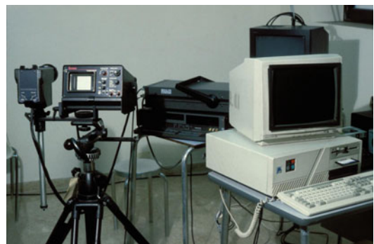
Fig. 11.1 A FLIR® thermographic camera provided by a PC for elaboration and storage of the IR images
