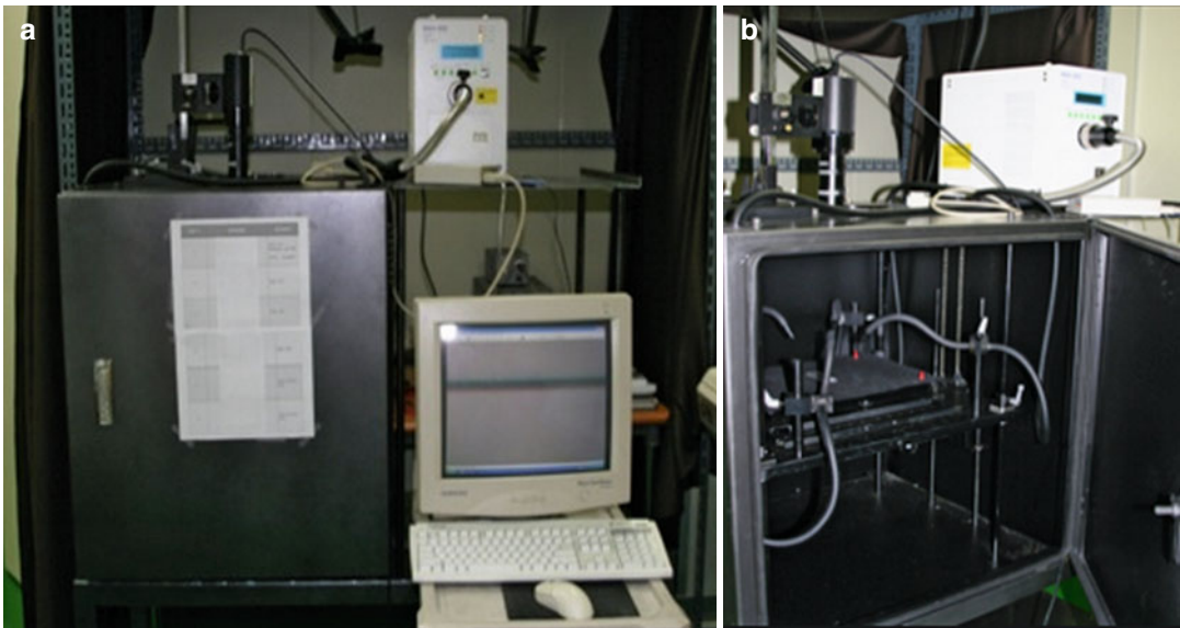
Fig. 41.2 The in vivo optical molecular imaging system that we created includes a xenon arc lamp (light source), multiple filter systems to detect specific excitation and emission spectra, and a cooled CCD detector. (a) Outer schematic diagram of the system and (b) inner schematic diagram of the system
