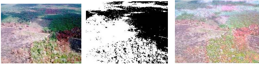
Fig. 7 (a) Aerial Image having cloud-shadows (b) Shadow extracted image (c) Shadow processed image
