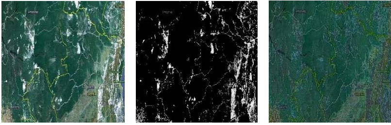
Fig. 6 (a) RGB Satellite Image (b) Cloud extracted image (c) Cloud processed image
