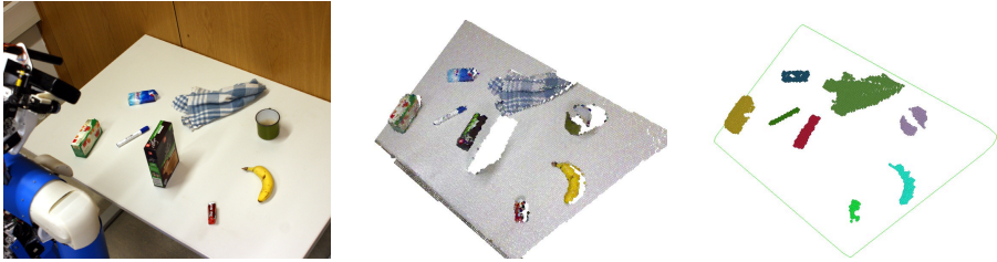
Fig. 2. Object detection. Left: example table top setting. Center: raw point cloud from the Kinect with RGB information. Right: each detected object is marked with a distinct color.
