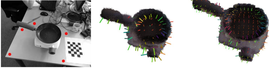
Fig. 4. Learning of object models. Left: during training the user selects points (red dots) to form a convex hull around the object. Center: color and shape distribution modeled at 5 cm resolution. Lines indicate surface normals (color-coded by orientation). Right: color and shape distribution modeled at 2.5 cm resolution.
