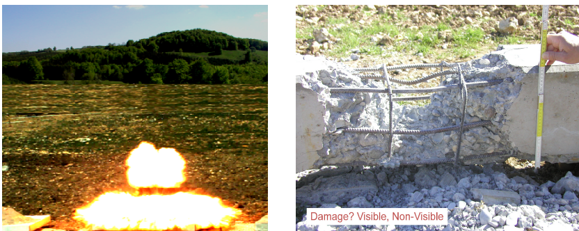
Fig. 5 Left: Contact detonation, ignition, right: column damaged
