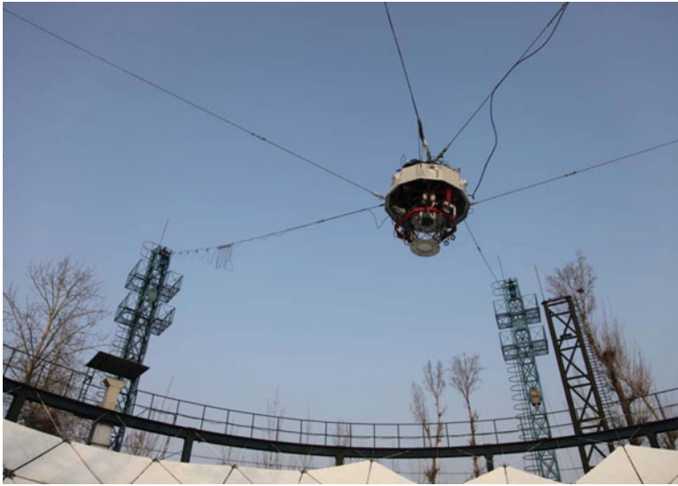
Fig. 4 40m diameter six-cable driven parallel manipulator
