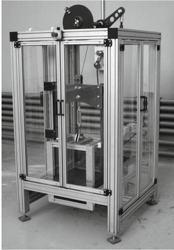
Fig. 4 CBOS testing machine for small rope diameters at the Institute of Mechanical Handling and Logistics, Stuttgart (IFT)
