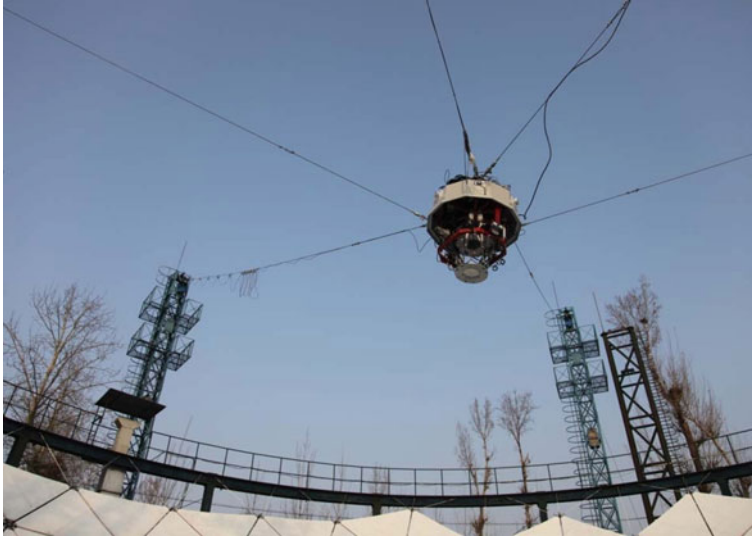
Fig. 4 40m diameter six-cable driven parallel manipulator
