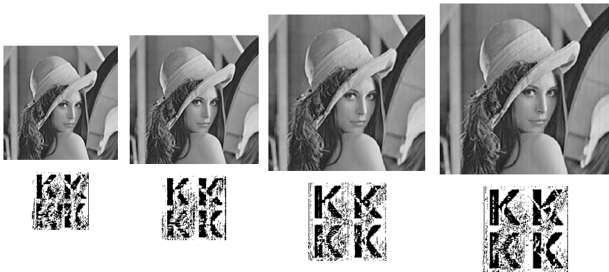
Fig. 12. Watermarks extracted from watermarked image scaled by multiplying ratios 0.8, 0.9, 1.1 and 1.2 (from left to right)
