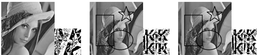
Fig. 14. Watermarked images and watermarks extracted from watermarked images subjected to several attacks (from the left, resizing & rotation & clipping, JPEG compression with compression ratio 25.25% & marking, and JPEG 2000 compression with compression ratio 10.81% & marking)
