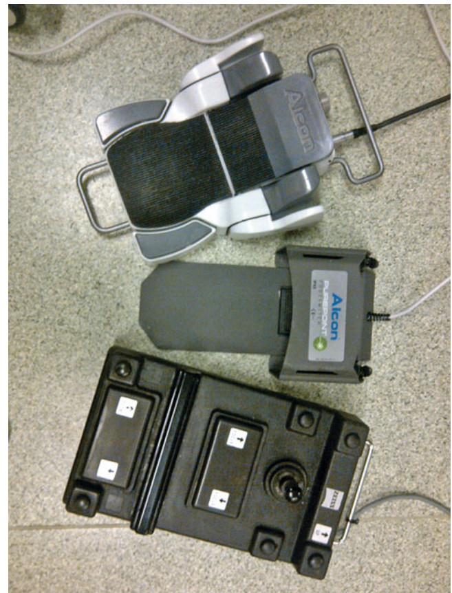
Fig. 2.2 A standard footpedal arrangement vitrectomy on left and microscope controls on the right. The laser controls in the centre can be worked with the left foot whilst using the microscope X/Y on the right
