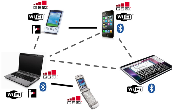
Fig. 1. An instance for 3MI represented by a set of devices connected according to their proximities and their available interfaces. The black full edges represent a possible solution for 3MI if they are correctly activated by means of suitable interfaces.
