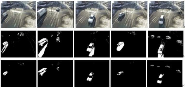
Fig. 19. Examples of car, first row is current image, second row is foreground image with shadow, third row is result
