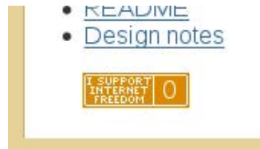
Fig. 1. Flash proxy badge on a web page. It runs in a visitor’s web browser, and the (optional) counter increments for each client served. Clicking on the badge disables it.
