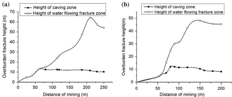
The maximum height of overburden water flowing fracture is 64.16, according to Chinese coal mine of preventing water regulation, 3 times of coal mining thickness should be added for security considerations. It will be dangerous for mining when the overburden thickness is thinner than 82.16 m, and the upper mining limit determined at elevation of -175 m (overburden height is 90 m) should be safe.
