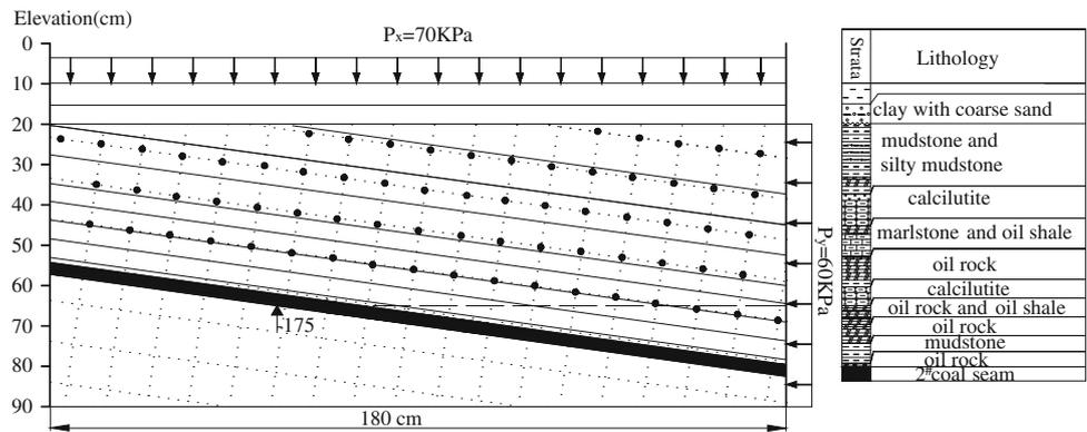
**Fig. 3** Overburden failure height with distance of mining
