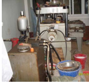
Fig. 2 The equipment used for the determination of tensile strength of the root of arbor
