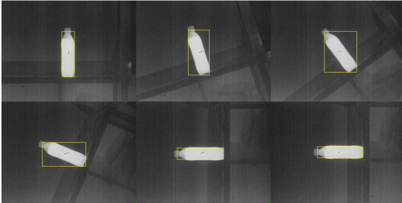
Fig. 6 Images acquired from thermal imaging camera during rotation by a roll angle
