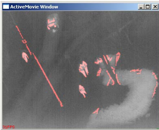
Fig. 16 Result of the blob detection algorithm on the sample IR video
