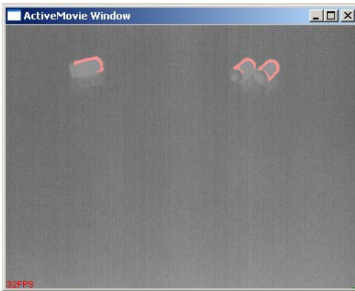
Fig. 14 Result of the blob detection algorithm on the sample IR video
