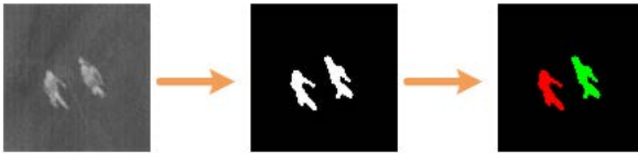
Fig. 1 Visualization of blob detection and blob labeling algorithm
