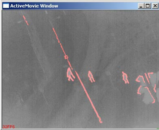
Fig. 15 Result of the blob detection algorithm on the sample IR video
