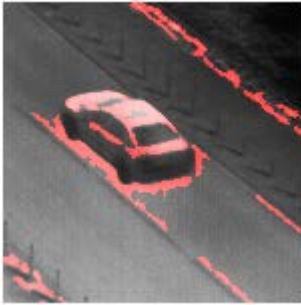
Fig. 20 Result of the blob detection algorithm on the sample IR video
