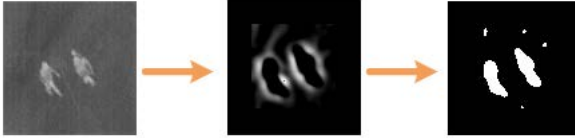
Fig. 8 Results of blob detection algorithm applied on sample real IR image
