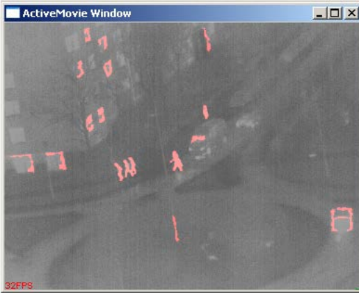
Fig. 17 Result of the blob detection algorithm on the sample IR video
