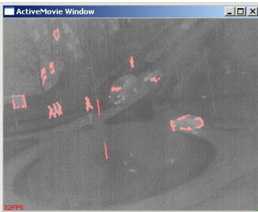
Fig. 18 Result of the blob detection algorithm on the sample IR video
