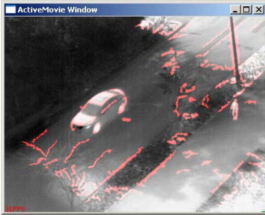
Fig. 19 Result of the blob detection algorithm on the sample IR video
