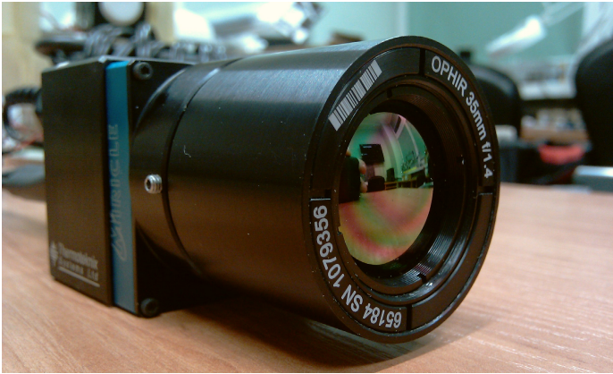
Fig. 3 A Thermoteknix 110K thermal imaging camera
