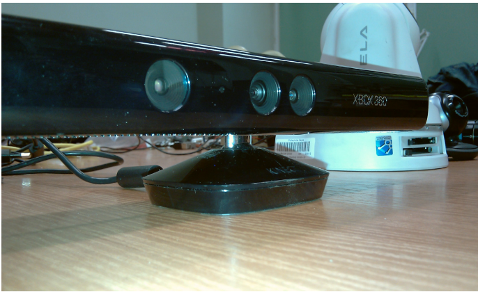
Fig. 4 A Microsoft Kinect game controller (RGB-D camera)
