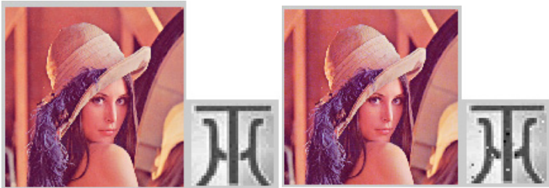
Fig. 4. Lena PSNR=34.2851, NC= 0.9978 : (a) original image and watermark, (b) watermarked image and extracted watermark
