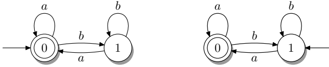
Fig. 1. Two hyper-minimal DFAs for the language (a^* + bb^*a)^* which are not isomorphic to each other; the symmetric difference of the languages accepted by these two DFAs is equal to the finite set \{\lambda\}
