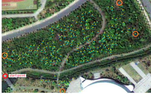
Fig. 5. In real GreenOrbs Testbed, 232 static sensors are deployed in a 200m \times 150m region. The 2D location coordinates of four boundary sensors are #1003 (8934.861,3103.606), #1153 (8763.517,3182.47), #744 (8850.326,3236.395) and #1193 (8958.139,3149.958), respectively.
