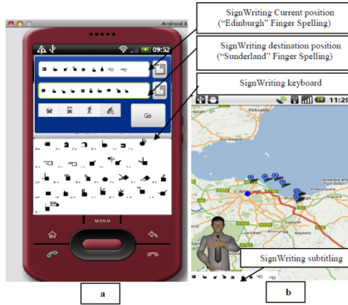
Fig. 3. (a) The SignWriting input interface (b) The route planner interpretation interface on the map
