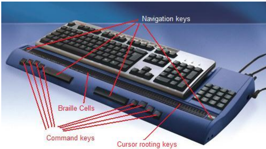
Fig. 1. Braille display with a set of control elements like Command keys, Cursor Rooting keys and Navigation keys
