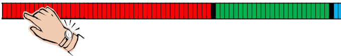
Fig. 3. Example of how a directory tree and a file list are presented on a Braille display in separate Braille frames
