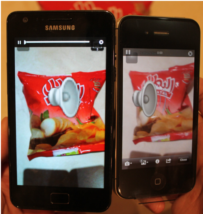
Fig. 2. The application running on Samsung Galaxy S II phone (left) and iPhone 4GS (right), the volume icon indicate that the object name is being spoken
