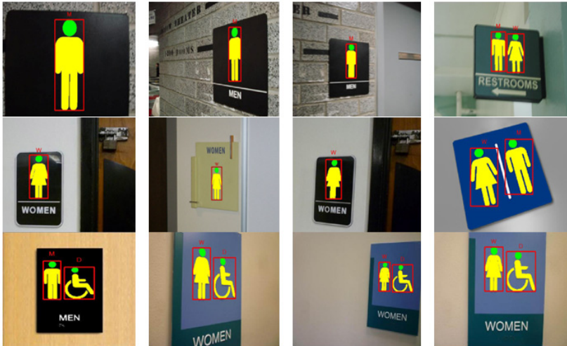
Fig. 4. Sample images with signage detection and recognition in our database include changes of illuminations, scale, rotation, camera view, and perspective projection, etc. The red boxes show the detected signage region, while the letter above each red box indicates the recognition of the signage: “W” for “Women”, “M” for “Men”, and “D” for “Disabled”.
