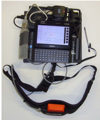
Fig. 1. Our navigation system. The combined accelerometer, magnetic field sensor and gyroscope can be seen on the strap.
