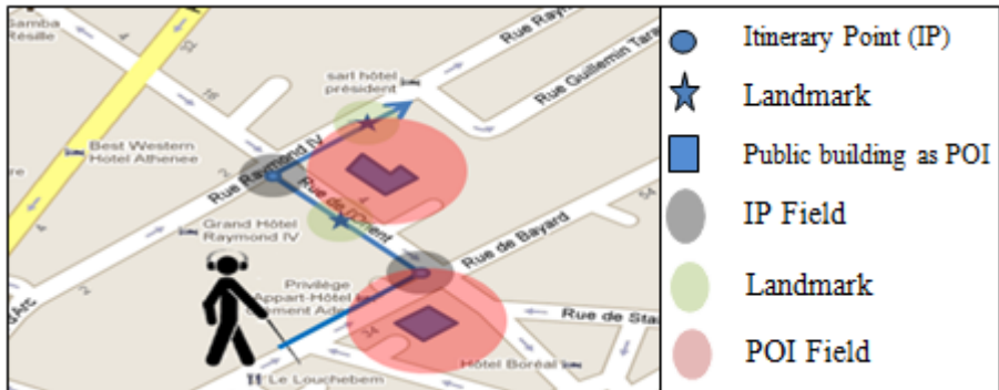
Fig. 2. Part of a selected route with Itinerary Points (IP - small circle), Points of Interest (POIs - squared shapes) and landmarks (stars) is represented. The activation field of IPs, POIs and landmarks are respectively figured in gray, red and green.
