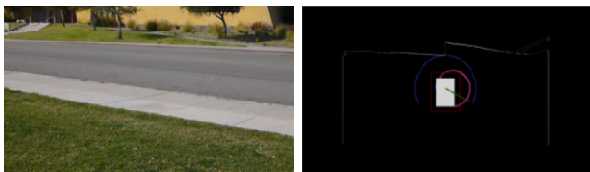
Fig. 5. The inclined LRF detecting and measuring the drop-off of a roadside curb
