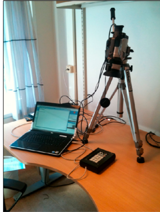
Fig. 3. Set up using video capture and the Morae usability software (Source: NR)
