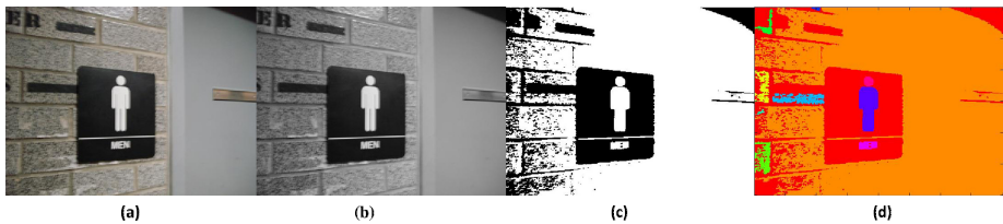
Fig. 2. Image Preprocessing for restroom signage detection. (a) Original image, (b) Gray image; (c) Binary image; (d) Labeled connected components.
