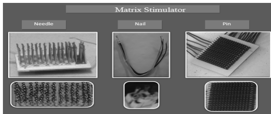
Fig. 1. Electrical Stimulation Matrix with different materials
