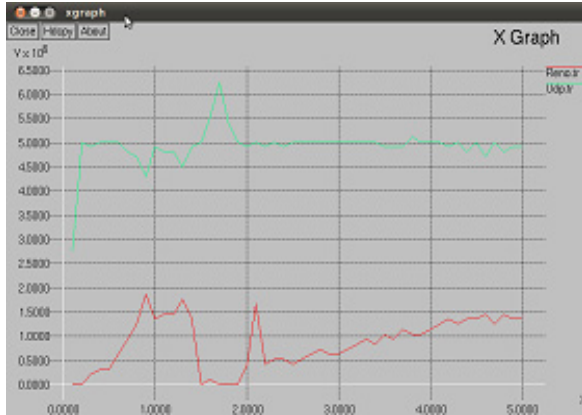
Fig. 4. The bandwidth usage of TCP Reno with 4Mb of UDP
