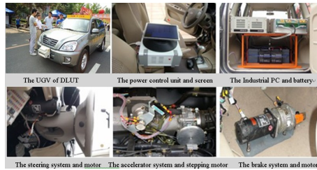
Fig. 1. The UGV's perception system and other refitted systems
