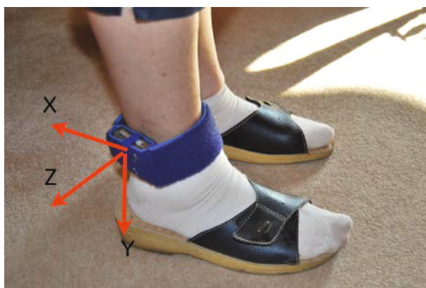
Fig. 1. The foot-mounted sensor worn by a volunteer. The bandage has a velcro closure and an opening for the sensor.
