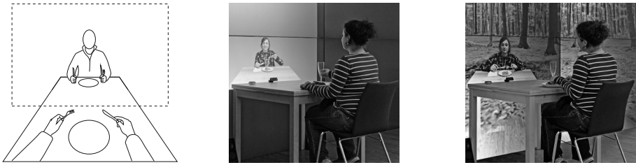
Fig. 2. System concept (left), person sitting in front of display wall, which is showing the video stream of the dining partner (center), and integration into virtual scene (right)
