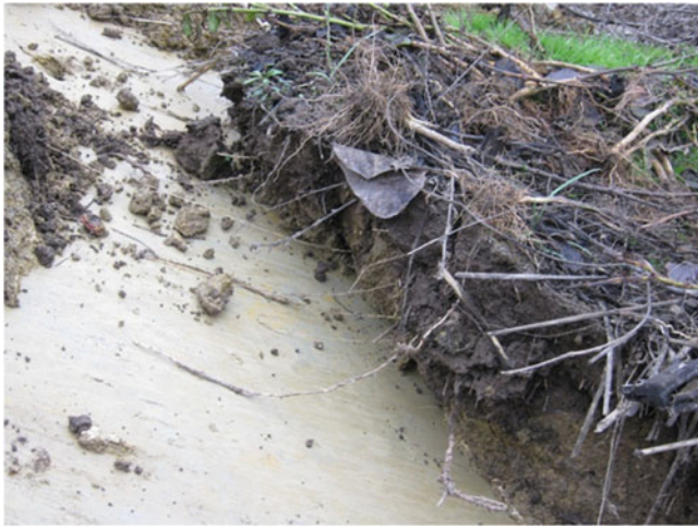
Fig. 9 Sliding surface (Photo December 2009)
