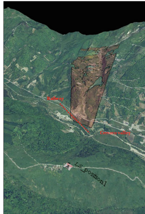
Fig. 2 The viewshed analysis for LS1 scan position with a range of 3 km
