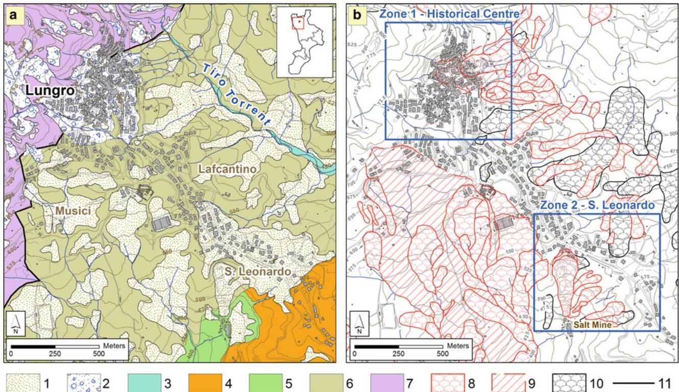
**Fig. 1** (a) Geological map of the study area: (1) detritical-colluvial cover (Holocene); (2) detritical carbonate deposits (Holocene); (3) alluvial deposits (Holocene); (4) middle Pliocene-Pleistocene succession; (5) Middle Tortonian-Messinian succession; (6) Diamante-Terranova
