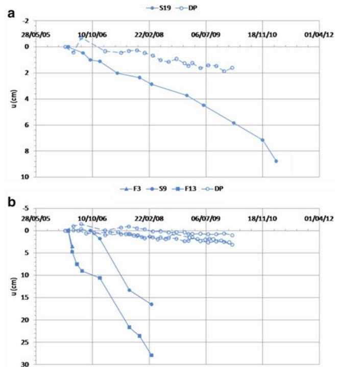
**Fig. 4** Trend of displacements measured from inclinometer (S19, F3, S9, F13) and DP (full-resolution DInSAR coherent pixel) along the satellite Line Of Sight (L.O.S.): (a) historical centre, (b) S. Leonardo
