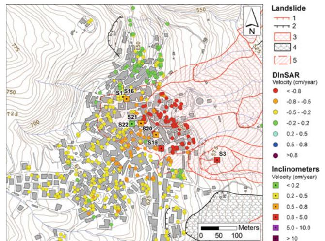
**Fig. 2** The historical centre: distribution of full-resolution DInSAR data and benchmarks equipped with inclinometers: (1) active main scarp; (2) dormant main scarp; (3) active slide-flow; (4) dormant slide-flow; (5) uncertain body of active landslide zone
