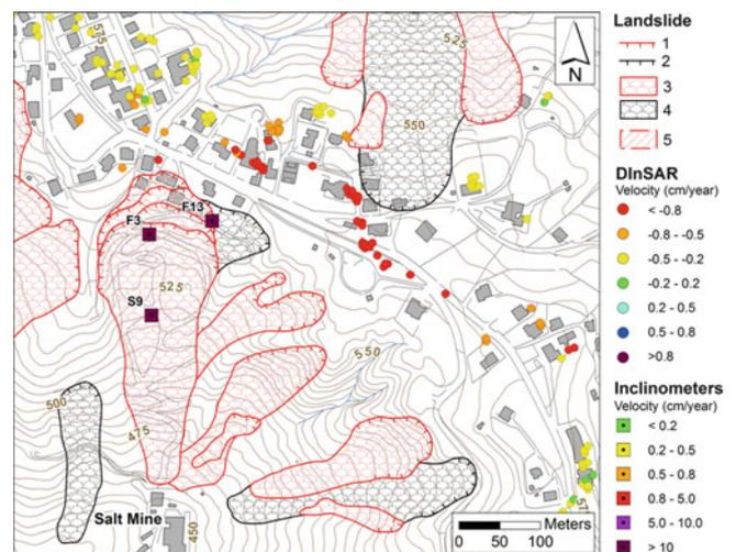
**Fig. 3** The S. Leonardo area: distribution of full-resolution DInSAR data and benchmarks equipped with inclinometers: (1) active main scarp; (2) dormant main scarp; (3) active slide-flow; (4) dormant slide-flow; (5) uncertain body of active landslide zone
