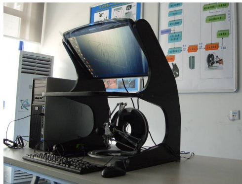
Fig. 3. The virtual reality force feedback haptic device (Omega.6, Force Dimension) and immersive workbench(Display Series 300, SenseGraphics)
