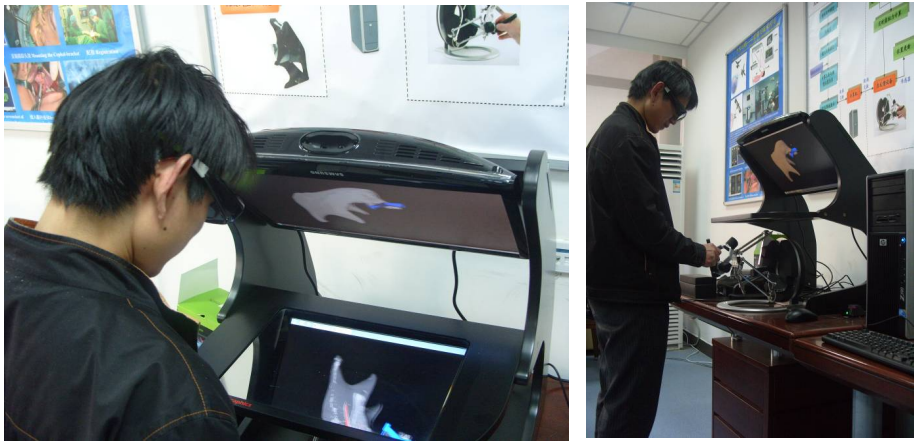
Fig. 5. The experiment of the virtual surgical training system with the force feedback haptic device and immersive workbench
