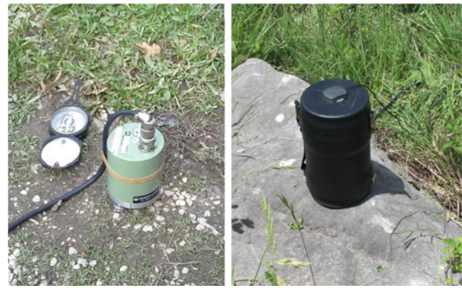
Fig. 1 Trillium Compact broad band seismometer placed on the ground ( left ) and under the insulating cover ( right )
