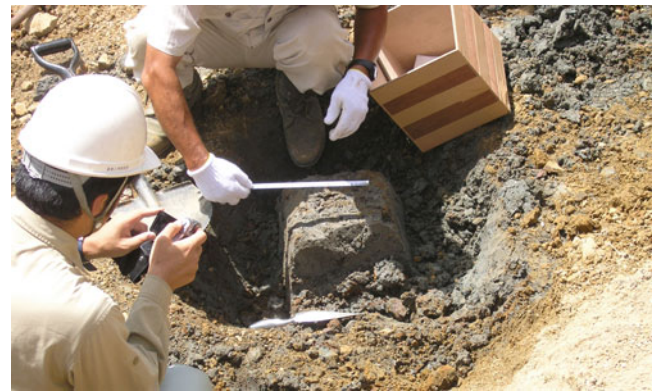
Photo 2 Undisturbed soil sampling at the lower surface of the slope
