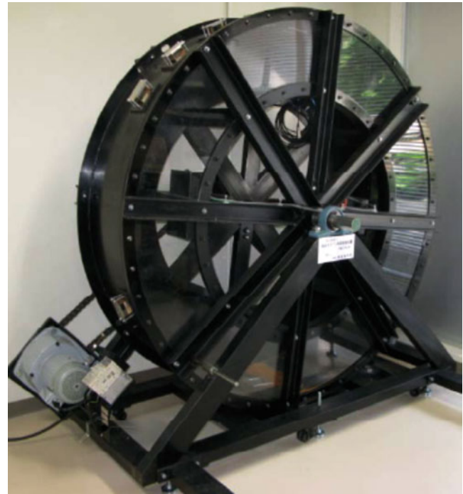
Fig. 1 Photo of the apparatus to simulate a submarine landslide and damage of a communication cable
