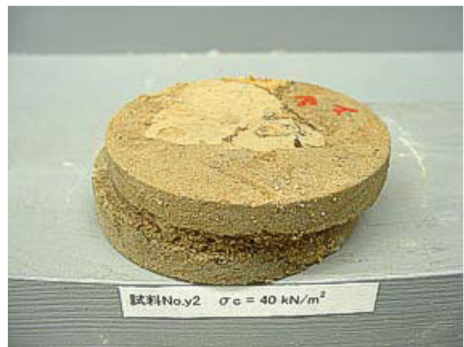
Fig. 5 Test specimen consisting of upper and lower silt rocks with tuff seam in between (This photo was taken after the test)
