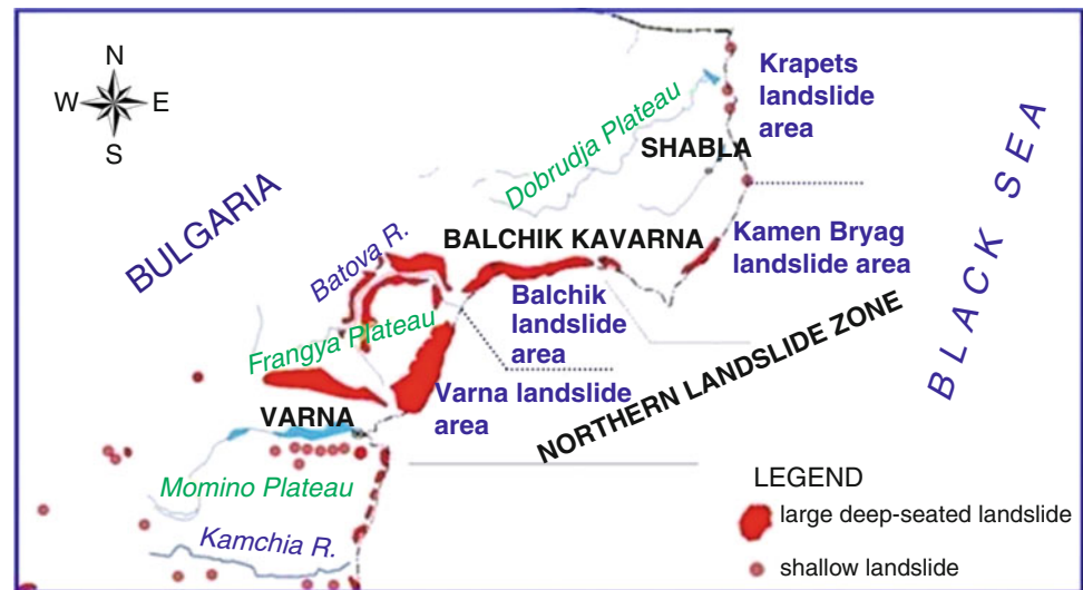
Fig. 1 Simple sketch of landslide areas along the North Bulgarian Black Sea coast
