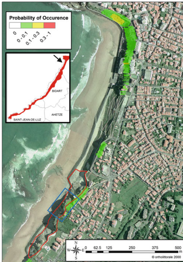
Fig. 10 Results of the modelling on the Côte des Basques cliffs. The most active area is highlighted by the red lining. The blue rectangle represents the localisation of Fig. 9
