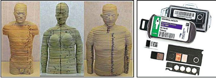
Fig. 9.5 The anthropomorphic phantom from the University of Florida ( left ), used by the author, and some OSL detectors ( right ). Photos from manufacturer's website
