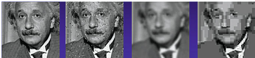
Fig. 9.10 Although each one of these images shows very different “noise” structures, they all produce the same standard deviation. Courtesy of Eduardo Guibelalde
