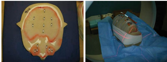
Fig. 9.5 The anthropomorphic phantom from the University of Florida ( left ), used by the author, and some OSL detectors ( right ). Photos from manufacturer's website
