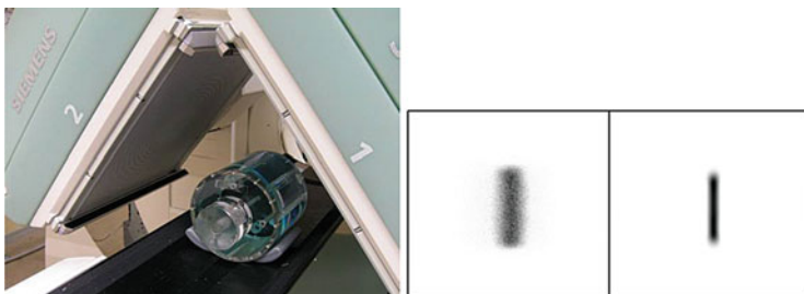
Fig. 9.14 (a) Experimental setup to measure the SPECT-reconstructed resolution in presence of scatter radiation [30]. A line source is placed inside the phantom made of PMMA. (b) Raw projection image of the line source. (c) Reconstructed sagittal slice
