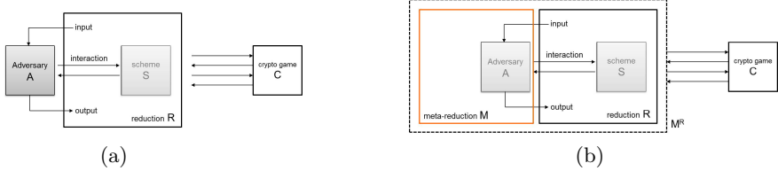
Fig. 1. (a) shows the reduction \mathcal{R} turning a successful adversary \mathcal{A} against scheme \mathcal{S} into a successful attacker \mathcal{R}^{\mathcal{A}} against a cryptographic game C , by simulating the scheme \mathcal{S} ; (b) shows the meta-reduction \mathcal{M} simulating the adversary \mathcal{A} and turning \mathcal{R} into a successful algorithm \mathcal{M}^{\mathcal{R}} against C directly
