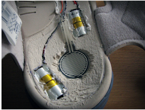
Fig. 1. Placement of a pressure sensor and two actuators in the heel of one sandal
