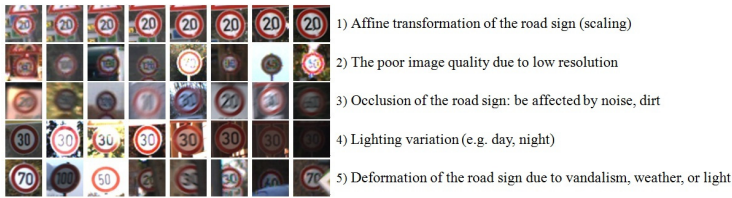
Fig. 1. Some representative difficult speed limit signs. All sample images are borrowed from GTSRB dataset.
