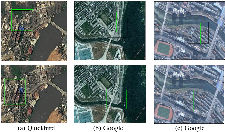
Fig. 3. The up row represents the matching results of mean-shift based on color diagram. The down row represents the matching results of mean-shift based on the gradient direction diagram. Aerial image in different places.
