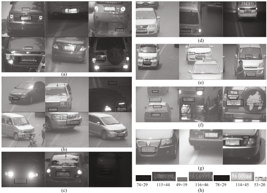
Fig. 6. Some example plate detections with variations in (a) illuminations, (b) view-points, (c) contrasts, (d) scales, (e) partial occlusions, (f) cluttered backgrounds, and (g) motion-blurs. Each black box shows the location of a detected license plate. (h) Some detected license plates upscaled for 3 times. The underneath of each plate image is its actual size.
