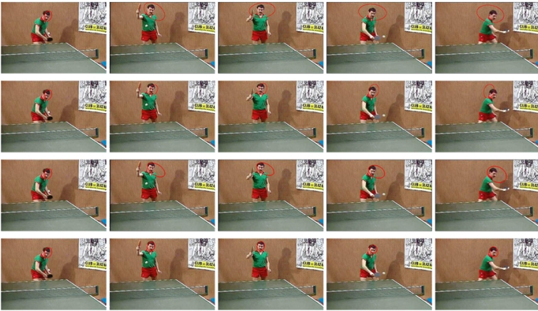
Fig. 4. Tracking the table tennis player sequence with inaccurate initialization. First row: EM-Shift. Second row: Mean Shift. Third row: SOAMST. Last row: the proposed method. From left to right, frames 0, 10, 20, 40 and 50 are shown.
