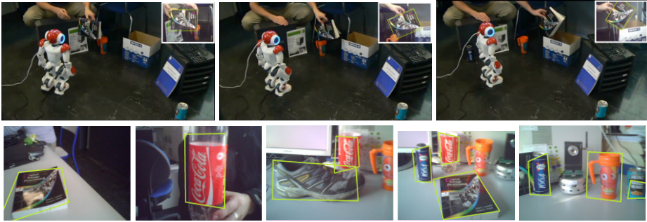
Fig. 10. Tracking a previously learned moving object (upper images: video http://www.youtube.com/watch?v=xxz3wm3L1pE ). The upper right corner of each image shows robot camera’s picture. The test’s results relative to a set objects’ detection by robot (lower images).
