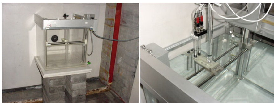
Fig. 13.10 Water phantom at WSU ( left ), with detail of paired ion chamber arrangement ( right )
