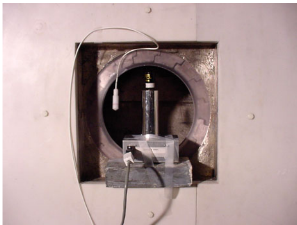
Fig. 13.13 RemSpec superheated nucleation spectrometer unit positioned in the source plane at WSU
