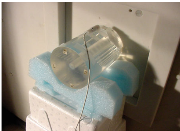
Fig. 13.7 Cylindrical PMMA phantom in the epithermal neutron beam at WSU. The diameter of the phantom is 12.5 cm and the length is 18.1 cm
