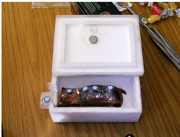
Fig. 13.12 Thermoluminescent dosimeters arranged on a hamster phantom used for preclinical BNCT radiobiological studies [46]
