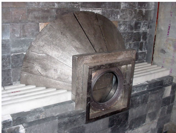
Fig. 13.4 Beam collimator installation at WSU showing the collimator with square exit port collar and lower borated polyethylene shielding
