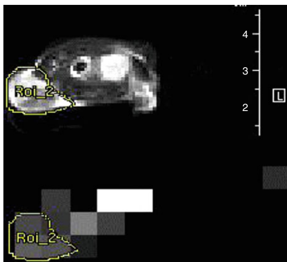
Fig. 12.1 The upper part is a conventional MRI showing a cross-sectional view through the lower abdominal region of a mouse. The lower part is a ^{10}\text{B} image shown on the same scale. The ^{10}\text{B} image is part of a 3D scan, obtained in 16 min with (6\text{ mm})^3 isotropic resolution, 2 h after injection of BSH into the mouse's tail vein. The ^{10}\text{B} distribution shows the highest accumulation in the bladder (upper right side of the anatomy). The average concentration in an implanted M2R mouse melanoma tumor (lower left part of the anatomy) corresponds to 27 ppm (Reproduced with permission from Bendel et al. [6])
