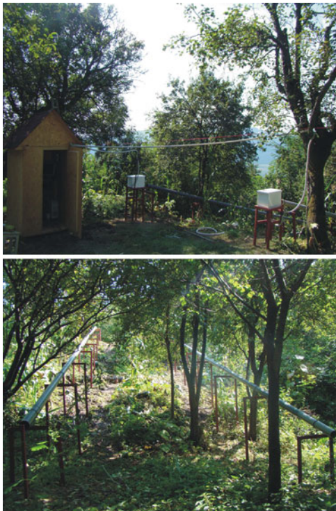
Fig. 7 The conventional extensometer and optical fiber sensor set-up at the landslide scarp (Maguricea landslide)
