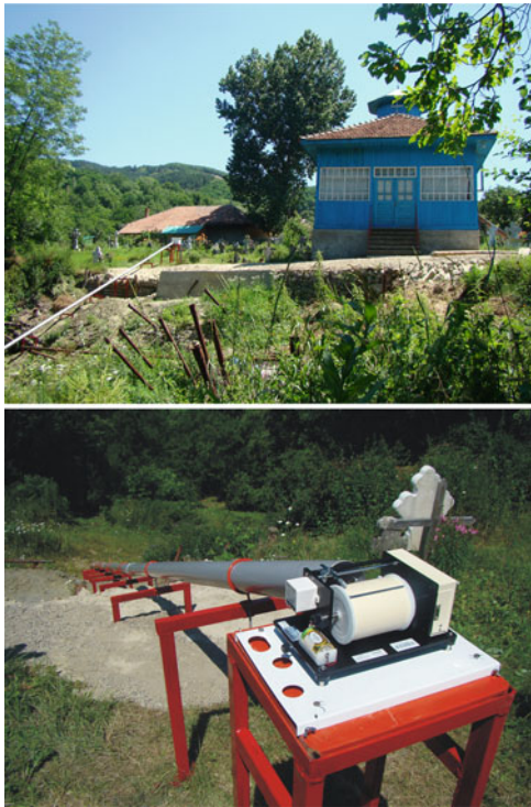
Fig. 6 The SRL-16 analog and digital extensometer placed across the landslide scarp which affects the entrance in the Colti church
