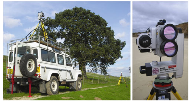
Fig. 3 The BGS Riegl LPM-i800HA laser scanner which can achieve an accuracy of \pm 15 mm
