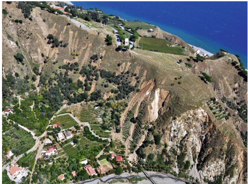
Fig. 1 Panoramic view of a slope affected by a pervasive series of mud/debris flows in the Briga catchment
