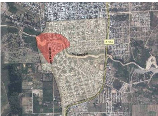
Fig. 10 The red polygon indicates the area most affected in the city, the light yellow area indicates how far the water and the solid material during flood went
