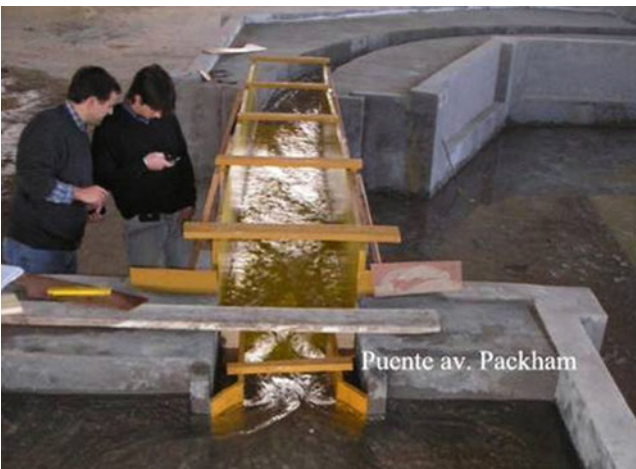
Fig. 6 Physical model at the National Water Institute – Argentina. Scale 1:40
