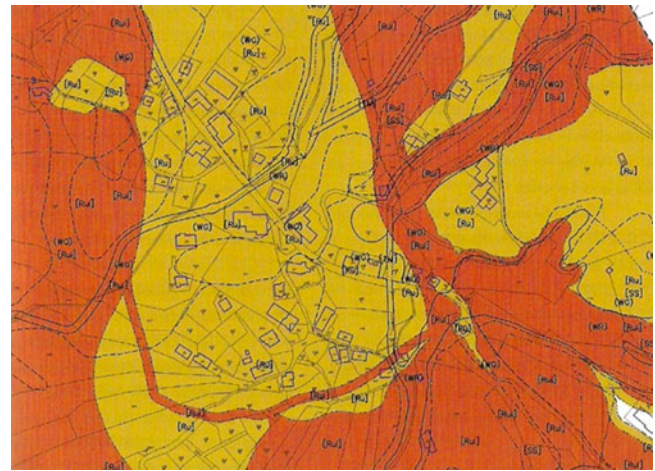
Fig. 2 Section of the hazard zone map of the community Sibratsgfall in Vorarlberg, with depiction of the brown reference areas
