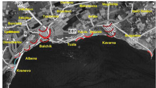
Fig. 3 Multi-risk map for Region 2. Hatched areas are seismic prone, lunar symbols – landslide (stonefalls) prone and light line – tsunami prone areas
