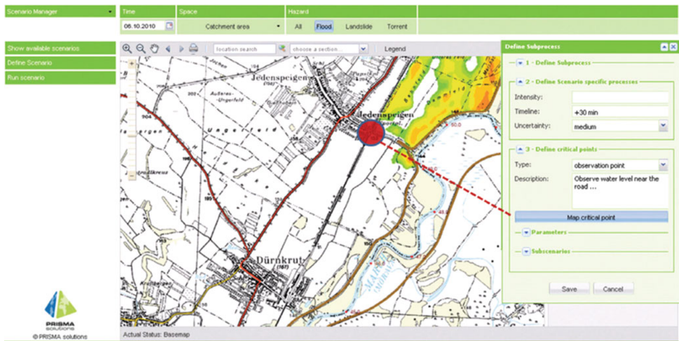
Fig. 7 CSA – Monitor II scenario manager supports the definition of observation points for further use in contingency planning
