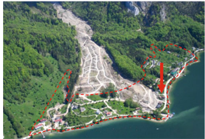
Fig. 4 Aerial photo of the landslide Gschlifgraben in May 2008. The red line marks the red hazard zone and the red arrow the main hazard area with five buildings and the local road (WLV GBL Bad Ischl)
