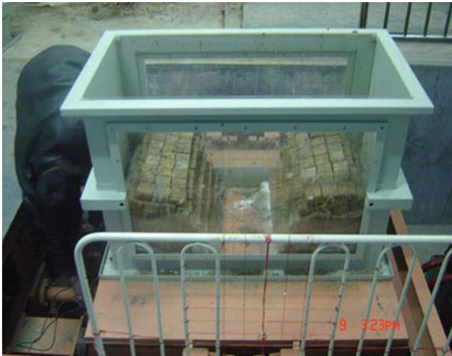
Picture 1 Model of block structure of bonding by the clay
