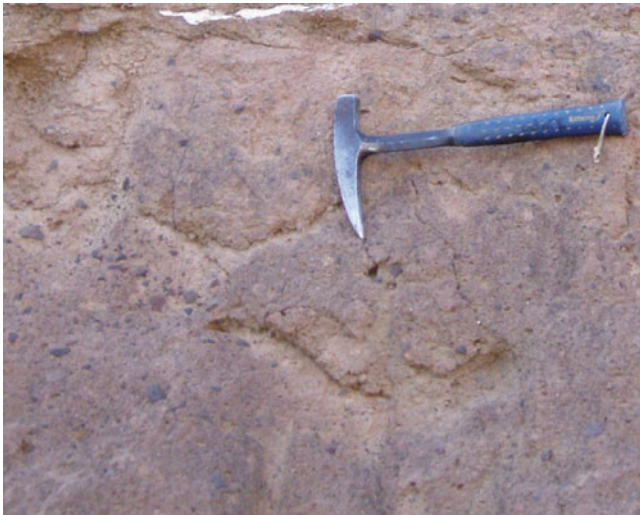
Fig. 6 Detailed view of the reddish non-welded ignimbrite. See Fig. 2 for site location
