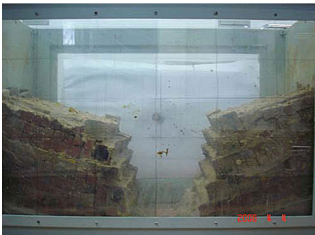
Picture 2 Model of slop dip toward excavation
