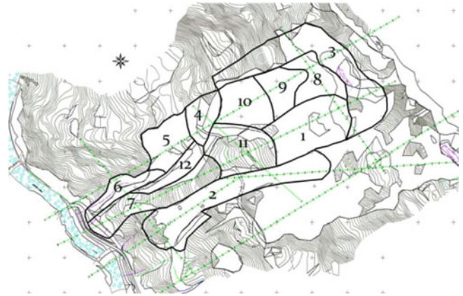
Fig. 5 Grohovo Landslide: 12 separate landslide bodies
