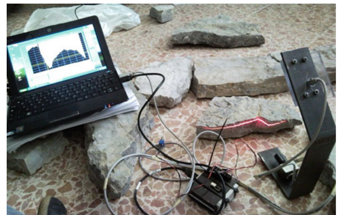
Fig. 2 A measurement stage: the profile is instantaneously printed on the netbook screen
