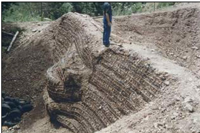
Fig. 2 Effect on downslope side of the reinforced embankment impacted during full-scale tests
