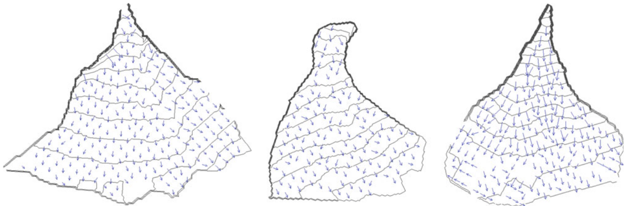
Fig. 2 G1 (e.g. Rio Fosse), G2 (e.g. Rio Saint Draia), G3 (e.g. Rio Secco) alluvial fan geometry plans. The increase of fan slope is shown by the arrow length (Tiranti 2008)
