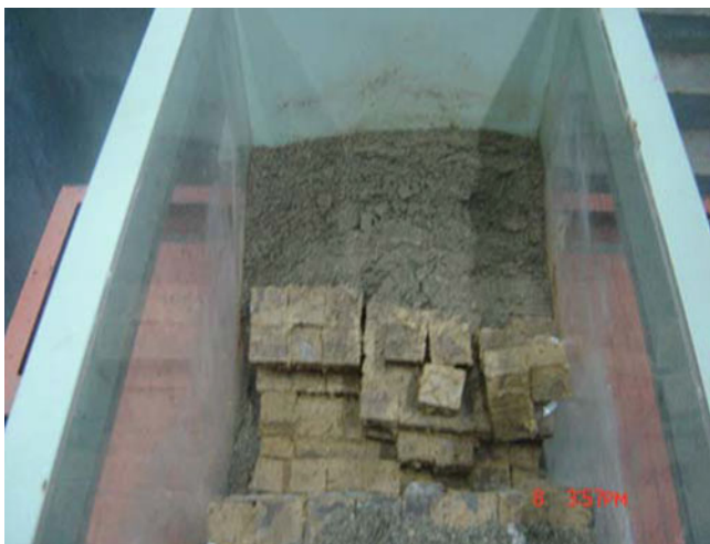
Picture 3 Third level sliding face destabilization occurs on the consequent slope
