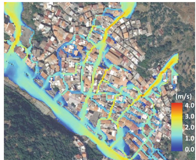
Fig. 9 Maximum velocity as observed for the scenario simulated with the TRENT2D
