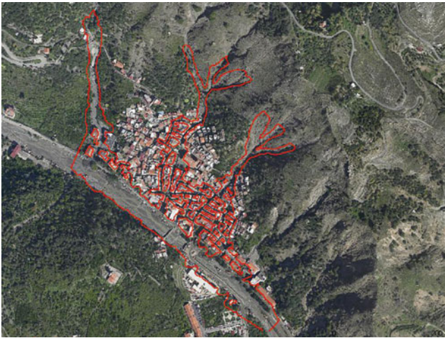
Fig. 3 Inundated area as observed for the scenario simulated with the FLO-2D
