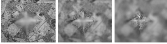
Fig. 2. From left to right the focus starts nearby (background in focus) and ends far away (imprint in focus)
