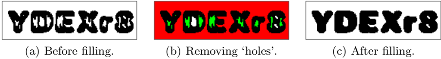
Fig. 11. Example of refining the extracted image by filling in the unwanted holes
